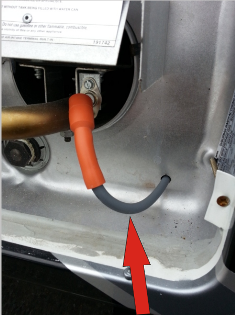
STEP 1. Replace Orange wire with suppression spark plug wire.
