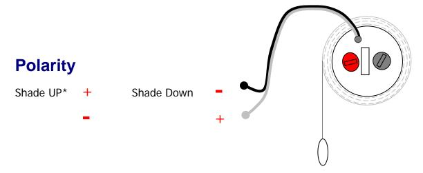
\*Note: The Polarity can change for special order systems such as reverse roll systems or systems where the motor is located on the right side. Standard systems always have the motor on the left side and are always wired as shown.
