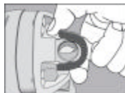
Step #1: Place your thumb at the edge of the clip as shown.
