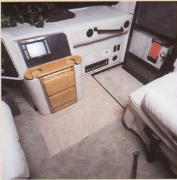
Air Driven Step Well Cover and Vinyl Tile Entry
